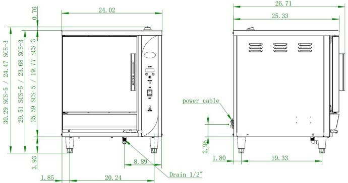
**NOTE:** Electrical Connection to Electrical Box: 1½" Conduit Connection w/9' of 1" Dia. BX Tube.
