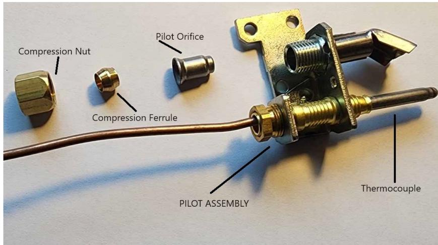
3. Remove the pilot orifice and replace it with the one that came in the kit.
