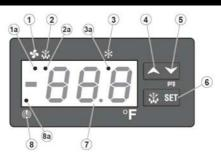
SET: ©To display target set point; in programming mode it selects a parameter or confirms an
