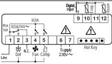
**NOTE:** The compressor relay is 8(3)A or 16(6)A according to the model. **120Vac supply:** connect to the terminals 6 and 7.
