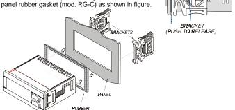
The temperature range allowed for correct operation is 0÷60 °C. Avoid places subject to strong vibrations, corrosive gases, excessive dirt or humidity. The same recommendations apply to probes. Let air circulate by the cooling holes.
