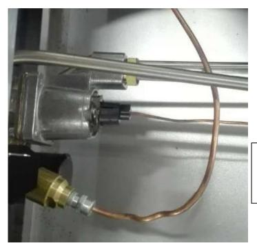
Install the Robertshaw thermocouple to the same position, Part # GR10075-2 (from Serial Date Code 1705) 3. Replace the pilot. Install this pilot with the new pilot mounting bracket. (shown below)
