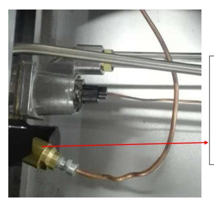
Remove this brass fitting on SABF valve and replace it with the brass fitting for Robertshaw thermocouple (Part # GR10020-1 thermocouple fitting, brass; screw thread: 11/32-32 & M15x1.
