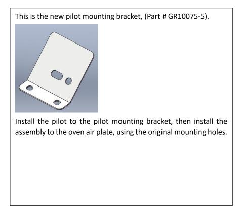
2. Install the pilot mounting bracket (w/pilot) to the original and same position as previous pilot assembly, then have the thermocouple installed.
