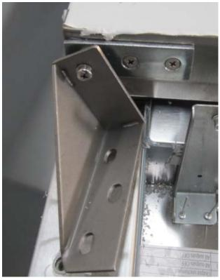
When you fix the hinges on to the door .The most important thing is ,the position of the Up Hinge should be like it shows on the picture, or the spring will not work .
