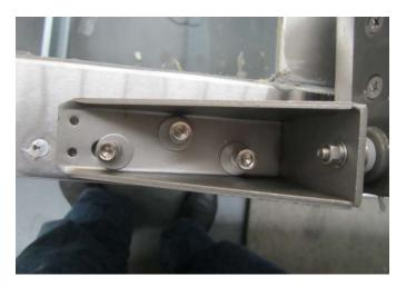
Be sure to when you fix the door on to the down hinge ,there should be two washer fixed on to the hinge.
