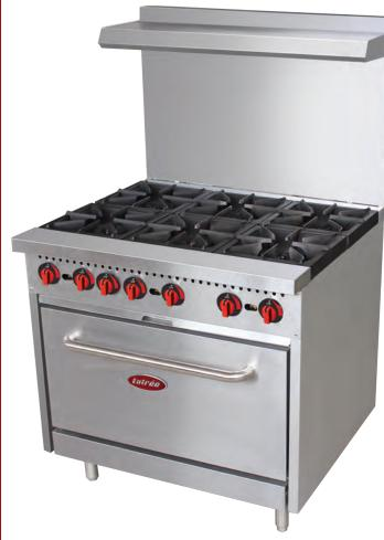
The Entrée Sauté Commercial Gas Range has powerful 30,000 BTU cast iron burners. Each burner has an individual pilot light - heavy duty 12" x 12" removable cast iron grate and individual instant light control knob. It is constructed with a stainless steel front and aluminized sides, 24.75" high backriser and shelf, 6" adjustable stainless steel legs or casters and a 3/4" NPT gas connection.
